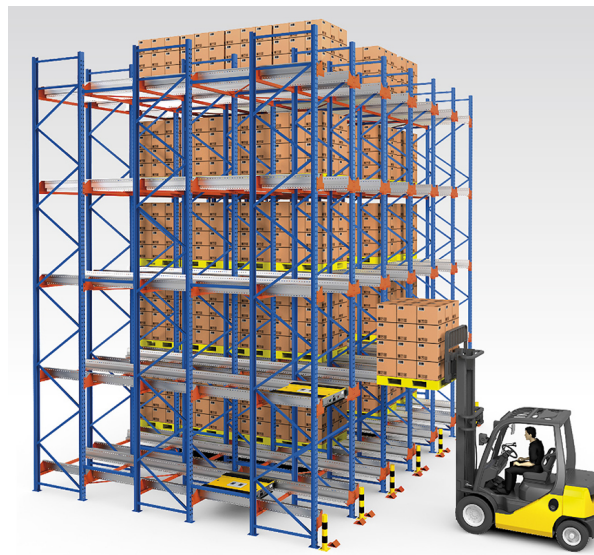
Figure B.8: Satellite and Shuttle Structure Example, [5]
